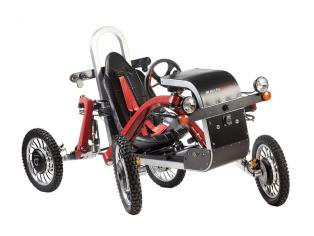
Four wheel steering on independent suspensions Four wheel drive- Engine brake and reverse gear 4.5 kWh battery (90Ah) integrated in the body frame (nacelle) Natural tilting when cornering Vertical correction on a slope F1 type steering wheel, steering column with lock All the controls are grouped around the steering wheel 4 Hydraulic disc brakes 220mm (8.7in) Accessible to all Designed and manufactured in France
